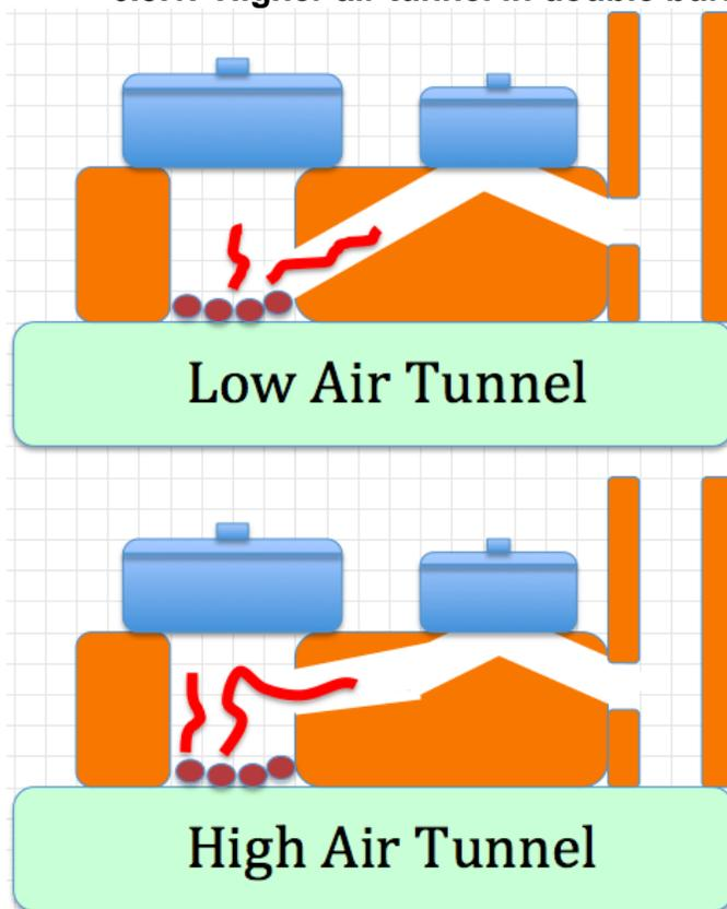
*Illustration 32: Higher air tunnel in double burner ICS*
