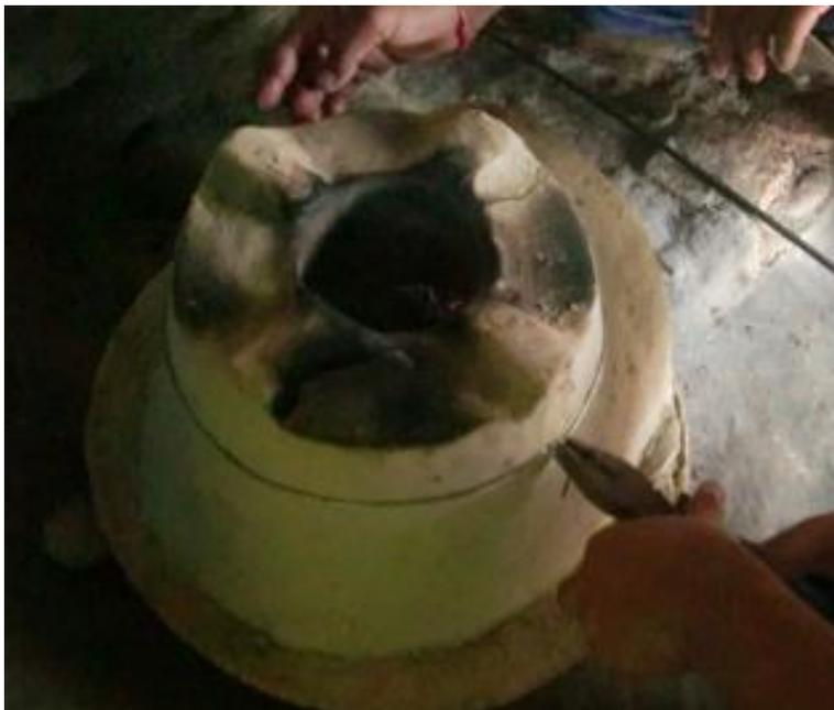
*Illustration 35: Using a metal wire to keep stove together after cracking*
